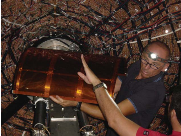
Figure 5: The AMADEUS carbon target (half cylinder) installed inside the Drift Chamber of KLOE detector in 2012.
