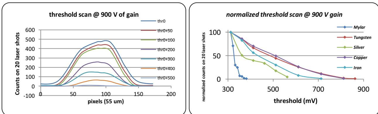
Figure 4: soft-X ray profiles at different thresholds (left) and threshold scan with different targets (right)
