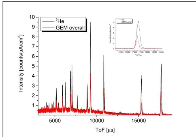
Figure 4: comparison between diffraction spectra obtained by an  $^3\text{He}$  tube and the GEM detector at  $90^\circ$  respect to the neutron beam on the INES beam line for a target of copper powder.
