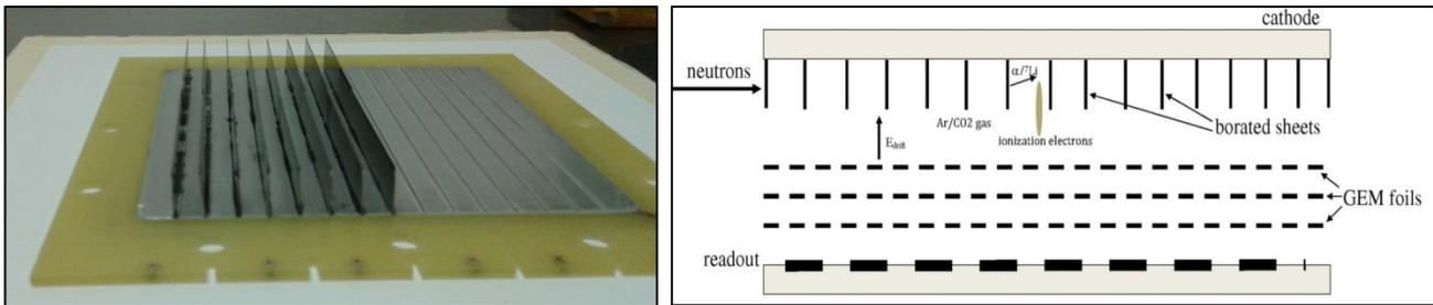
Figure 4:  $\text{B}_4\text{C}$  deposited silicon lamellae during the construction of the new GEM detector, a lateral layout of the side-on detector (right).
