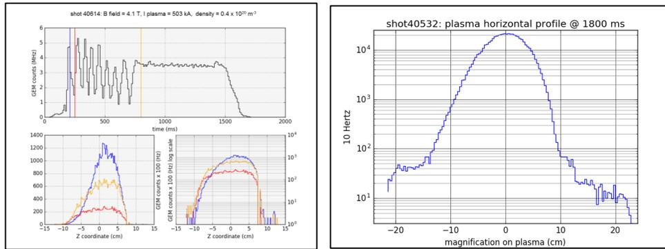
Figure 1: the observed temporal trace observed on FTU at 100 Hz of frame rate and the observed profiles at different times from the shot start (left), a measured 1D profile on an intense FTU shot showing the high dynamic range of the GEM detector (right)
