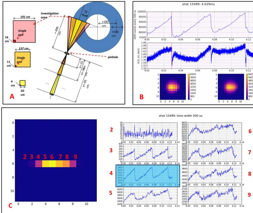
Figure 2: A) the observed areas when the distance between detector and pin-hole is changed. B) a comparison of ELM oscillation between GEM and an Electron Cyclotron Emission (ECE) measured. C) observation of the ELM oscillations.
