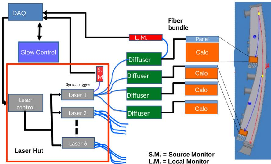
Figure 1: Schematic view of the Laser Calibration System design.
