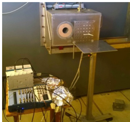
Figure 3: The collimated output of the TRIGA thermal column.
