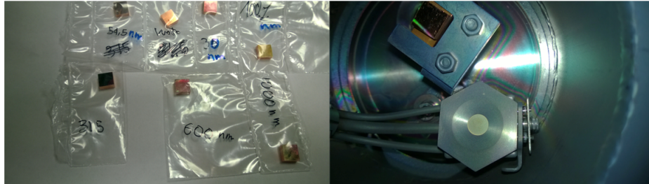
Figure 4: Left: photograph of some samples of \text{MoO}_3 films growth on flat copper substrates and sealed in plastic bags after deposition; right: photograph of the sample on the evaporation HV chamber with the thickness gauge.
