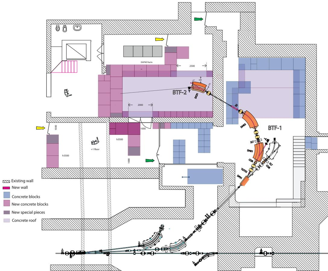
Figure 7: The new BTF layout with two beam-lines and two experimental areas.
