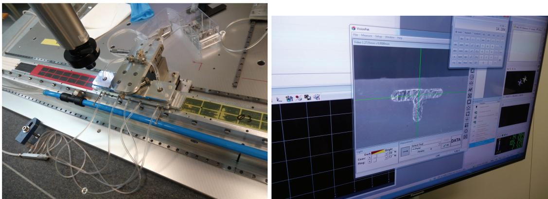
Figure 5: *The left panel shows one carbon fiber Cold Plate on the vacuum base with one glued module and a second one being placed: the carriage holds via vacuum another fiber glass module to be glued on the Cold Plate. A gluing mask (to be removed once the glue is dispensed) is also visible. The right panel show a detail for the marker of the fiber glass dummies as seen from the CMM camera. The dimensions of the marker are  $\sim 100 \mu\text{m}$ .*
