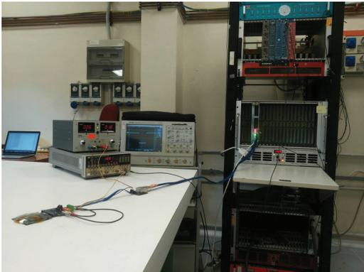
Figure 9: Test setup for the read-out of the  $pALPIDE4$  chip at the LNF. The single chip carrier board is interfaced to the MO-SAIC VME system which is in turn controlled by a Linux computer.
