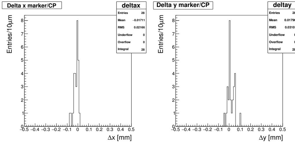
Figure 8: Left panel: distribution of the differences between the nominal and the measured marker positions along the  $x$  (short) direction (dimension) of the Half Stave. The right panel shows the same for the  $y$  (long) direction (dimension).
