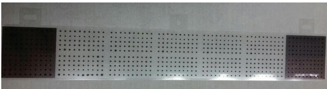
Figure 6: *The picture shows the Mylar dummy HIC. The four pad chips are visible at the corners.*
