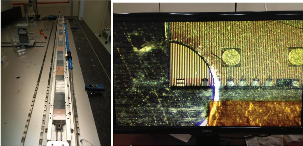
Figure 7: *The left picture shows an aligned HS locked by vacuum on the assembly base. The glued Mylar dummy modules are visible. The right picture shows a magnification of one dummy HIC pad chip at corner, where the reference marker of  $5\ \mu\text{m}$  size is clearly visible.*
