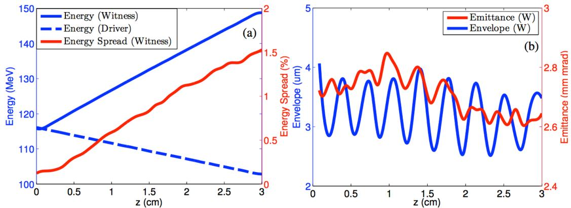
**Figure 2: Beam evolution along the capillary: (a) Energy gain and witness energy spread; (b) envelope (blue) and emittance (red) of the witness bunch.**
