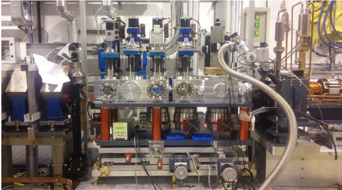
**Figure 3: PWFA chamber installed at the end of the linac.**
