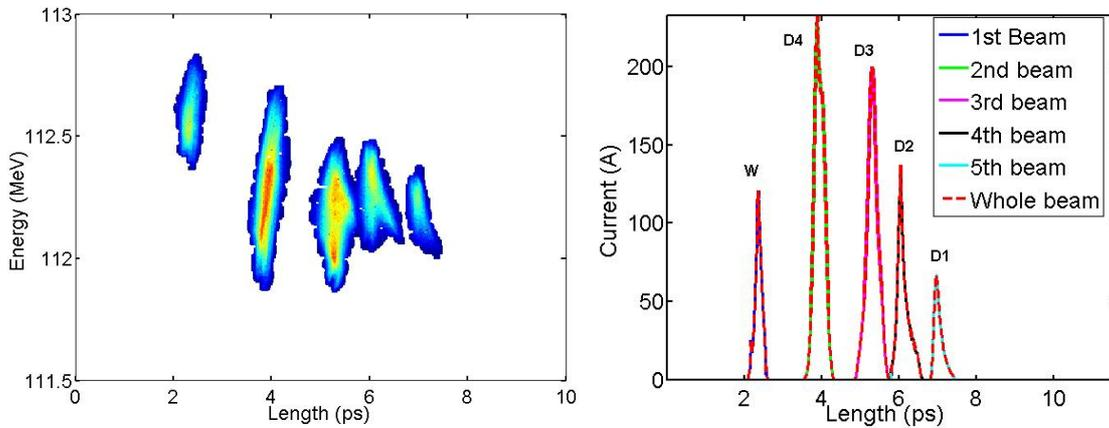
**Figure 1: Longitudinal phase space (left) and current distribution (right) for the 4 ramp drivers and 1 witness beam.**
