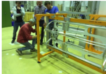
Figure 4: The STT mechanical frame prototype, during the installation at the Jülich FZ.
