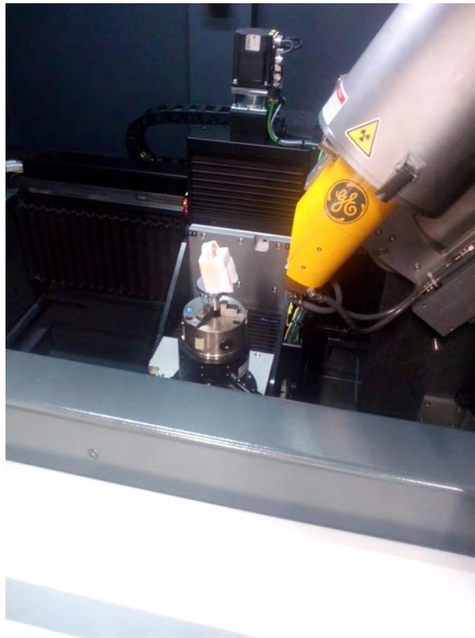
Figure 5: Photograph of the copper iris of a high-gradient cell installed on the sample holder for the X-ray CT scan to investigate the induced internal damage of components undergoing high-gradients (courtesy Labormet Due).
