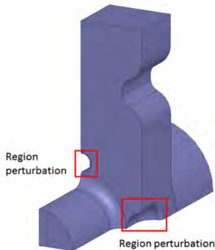
Figure 1: A quarter geometry of the improved TM01 mode launcher for quadrupole components minimization. The two perturbations are located between the rectangular waveguide and the smaller pipe.
