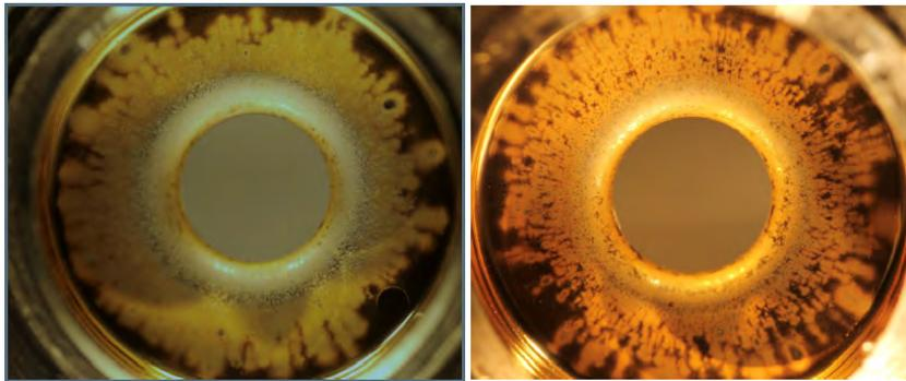
Figure 3: Images of the autopsy of an electroformed three cells Au structure: left) the image of the high gradient side of the center cell; right) the image of the high gradient side of the end cell. The removal of Au from the surface due to multiple breakdowns is evident in the region of the highest-electric field.
