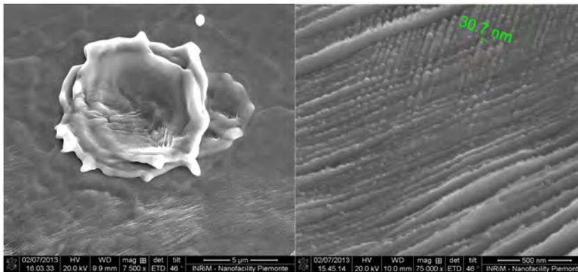
Figure 4: Details of the surface of a cavity exposed at SLAC (courtesy of V. Dolgashev). left) an isolated defect consisting in a molten Cu crater showing the texture ascribed to thermal fatigue; right) a magnified view of texture at the nanometer scale induced by the cyclic pulsed heating.
