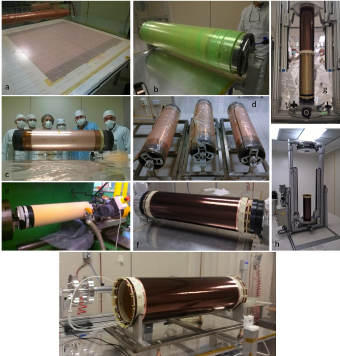
Figure 3: A summary of the construction: planar gluing of two GEM foils (a), the vacuum bag technique applied for the cylindrical gluing (b), a completed cylindrical GEM (c), the three CGEM used for the prototype (d), the machining of the rohacell surface for the cathode construction (e), the readout with its ground plane (f), the removing of the anode from its mould on the machine (g) the machine rotated of  $180^\circ$  (h), finally the detector completed and under test (i).
