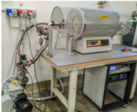
Figure 2: Picture of the CVD furnace. The main features of the system are: 3-zone temperature controller reaching 1200 °C; 3-inches quartz worktube connected to the gas distribution panel containing 3 gas flow controllers at one end, and to a rotary pump and to high-precision absolute-pressure reader at the other end.
