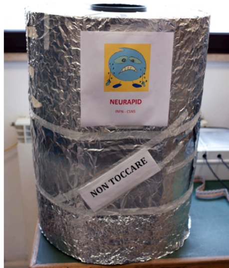
Fig. 19. The CYSP exposed to the vertical component of the cosmic-ray-induced neutron field at SVIRCO, Roma 3.
