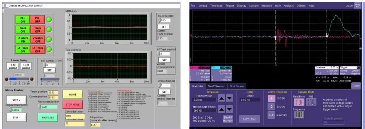
Figure 6: a) control window of PLL of the 2 lasers; b) Screenshot of signals induced by the electron and photon pulses passing near the IP
