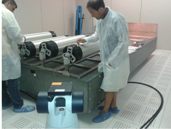
Figure 2: The laser measurement of the 5 Al molds. The laser head is shown in front
