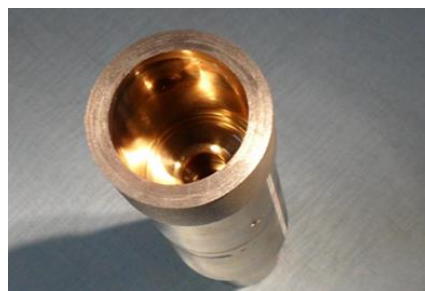
a) Final X-band structure (left picture) and its cross section (right picture) after removal of mandrel
