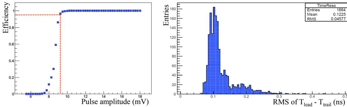
Figure 6: *Left: threshold profile. Right: distribution of the RMS of repeated time measurements of a probe signal, performed with every channel. The probe signal has an amplitude of 100 mV and a fixed width of 30 ns to within 40 ps RMS.*
