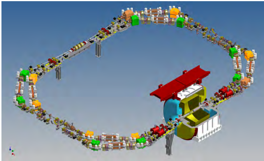
Figure 1: The DAΦNE Main Rings in the present crab-waist scheme for the KLOE-2 run.
