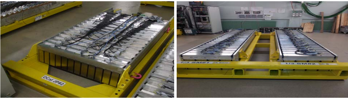
Figure 8: Left: picture of 1 full DCal super-module. Right: photo of the 2 reduced DCal super-modules.
