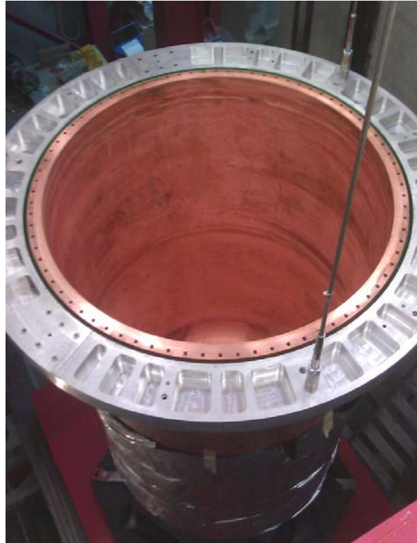
CUORE: installation of cryostat Outer Vacuum Vessel @LNGS
