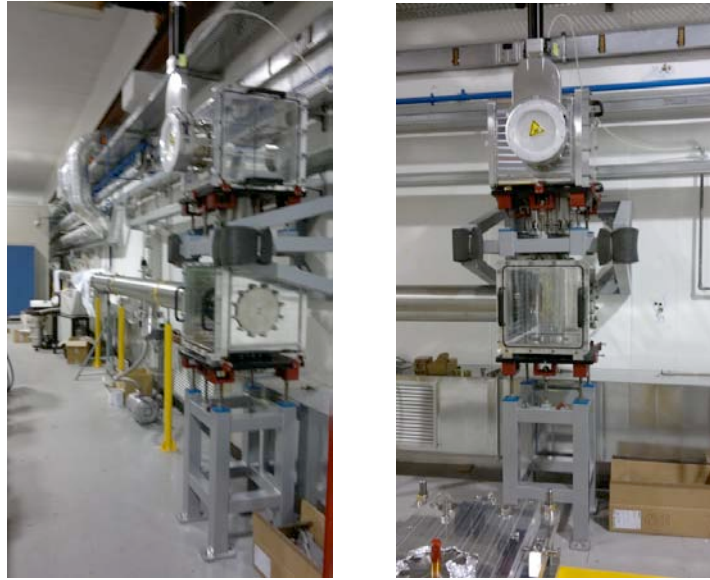
Figure 4.6: SL-Thomson laser transfer lines inside the SPARC bunker (left). Motorized mirror vacuum chamber (right).
