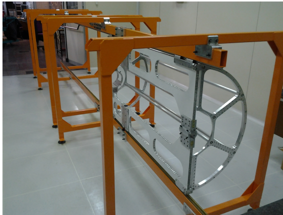
Figure 4: The prototype of the Central Tracker mechanics hold by the insertion support system.
