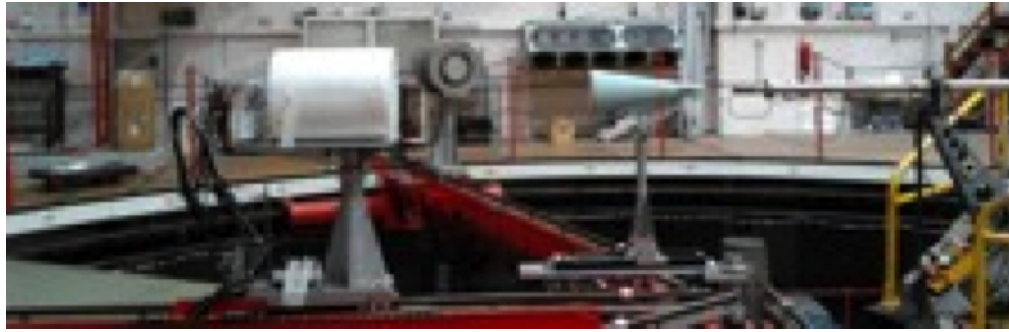
Fig. 10: On the left: moderating cylinder embedding seven ATNDs simultaneously acquired. On the right: shadow-cone used for room-scatter subtraction purposes at the NPL reference monochromatic neutron beam facility.
