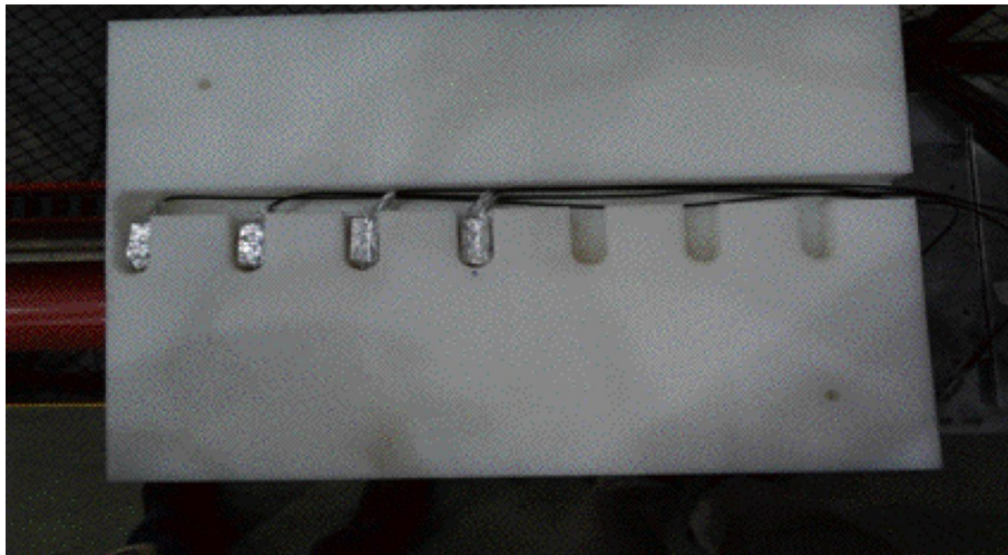
Fig. 12: Cross section of the testing cylinder (50 cm length, 40 cm diameter). Position 1 is the shallowest one, whilst position 7 is the deepest one.
