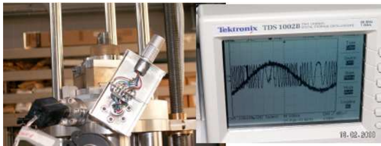
Figure 1: (left) The RF filter box of the SQUID connector; (right) SQUID test performed at 4.2K with an a.c. magnetic field of 0.012G at 107Hz. 15 fluxons quanta have been measured
