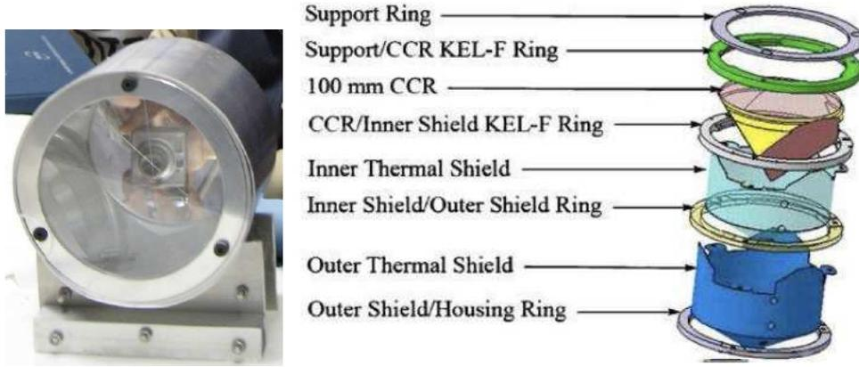
Figure 3: Views of current design of the MoonLIGHT/LLRRA21 CCR: (a) fully assembled; (b) exploded view with its internal mounting elements and outer aluminum housing.
