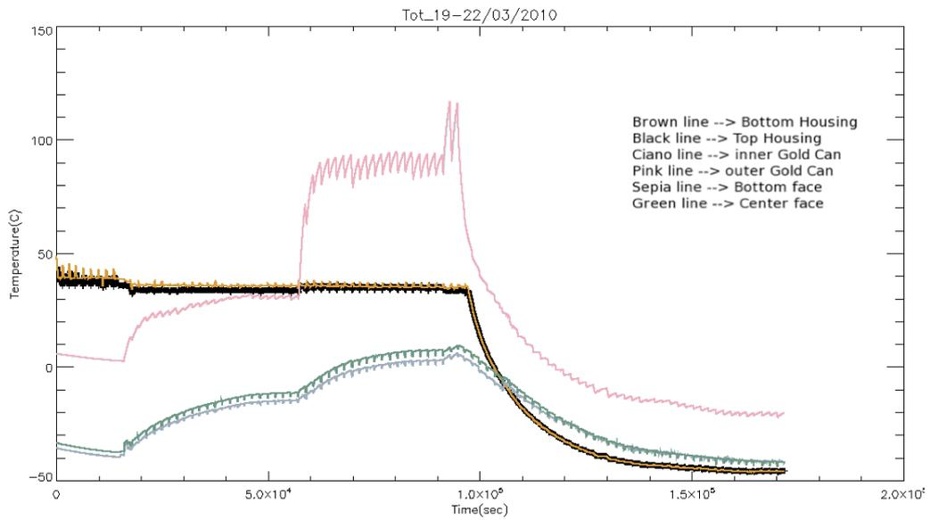
Figure 8: MoonLIGHT/LLRRA-21 flight CCR temperature variations of various housing parts and of CCR (19-22/March/2010).
