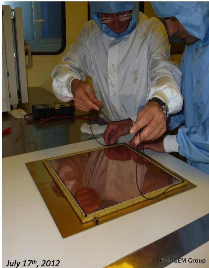
Figure 3: Assembly of a GEM detector.
