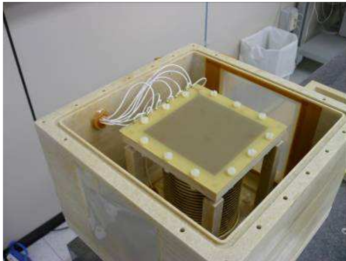
Figure 6: The TPC-GEM prototype
