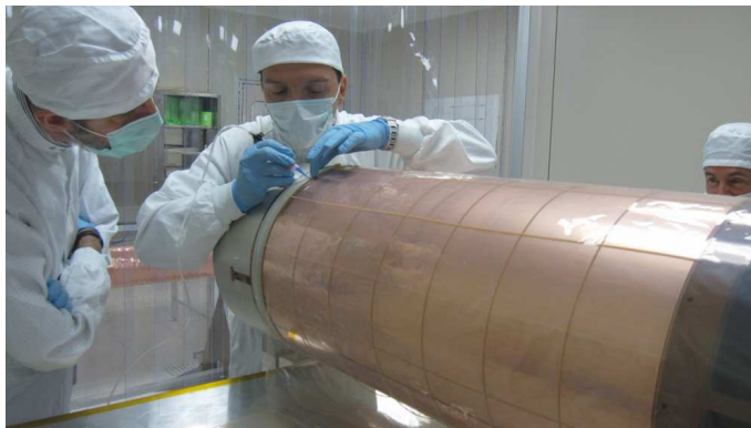
Figure 2: The PEEK grid is fixed on the kapton outside the GEM foil active area with epoxy glue.
