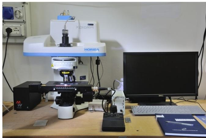
Figure 7: The new micro-Raman instrument XPLORA from Horiba Jobin-Yvon installed in 2012.
