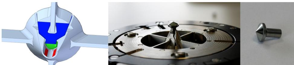
Figure 1: Design and realization of the dedicated ATR objective with a removable Germanium crystal tip.
