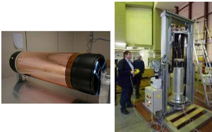
Figure 6: *Left: The aluminum moulds used for the construction of the cylindrical electrodes of the inner tracker. Right: The assembly machine (Clessidra) used for the insertion of the cylindrical electrodes one into the other.*
