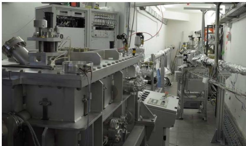
Figure 9: *The HEB beamline under construction with the recently mounted PGM monochromator on the left side.*
