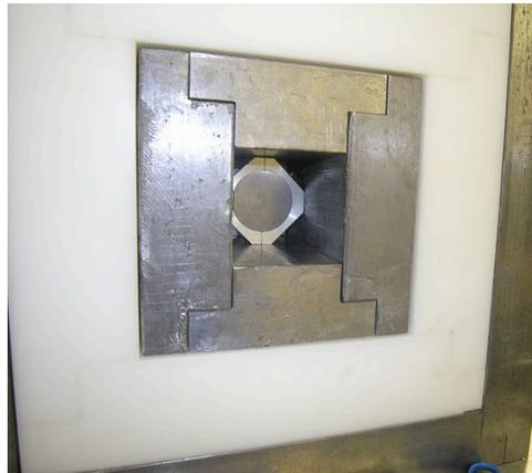
Figure 2: *Target located inside the shielding apparatus.*
