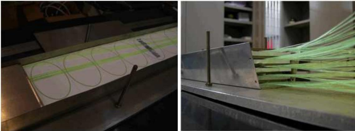
Figure 7: *The full-scale prototype of one module of the QCALT calorimeter, with the tiles assembled and the fibers for the transport of the light to the readout end side.*
