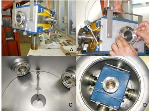
Figure 1: *Photographs of the PRESS-MAG-O cryostat during the reassembling operations of the optical lines of the superconducting magnet.*
