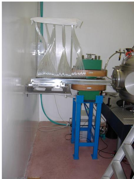
Figure 19: The Magnetic Spectrometer of SITE.
