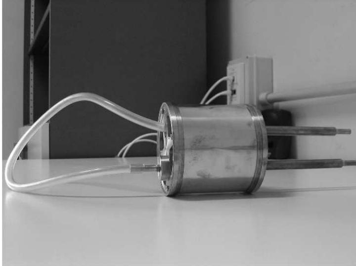
Figure 1: *The VIP copper target.*
