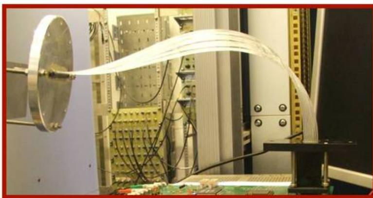
Figure 16: *Prototype of the fiber detector of the electron spectrometer of SITE.*
