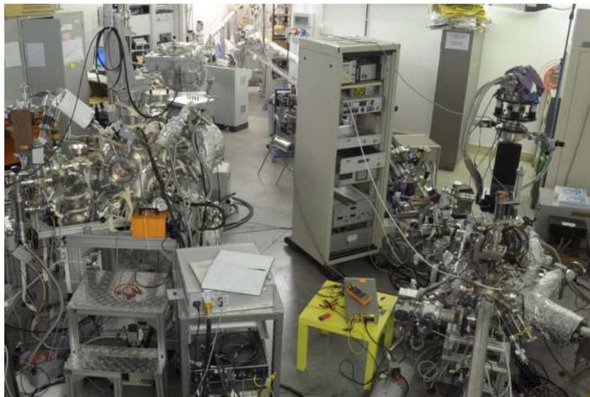
Figure 8: *Overview of the XUV DAΦNE-L laboratory. On the right side: the LEB beamline and (in front) its experimental chamber. On the left side: the HEB beamline under construction with the recently mounted PGM monochromator, and the experimental set-up.*
