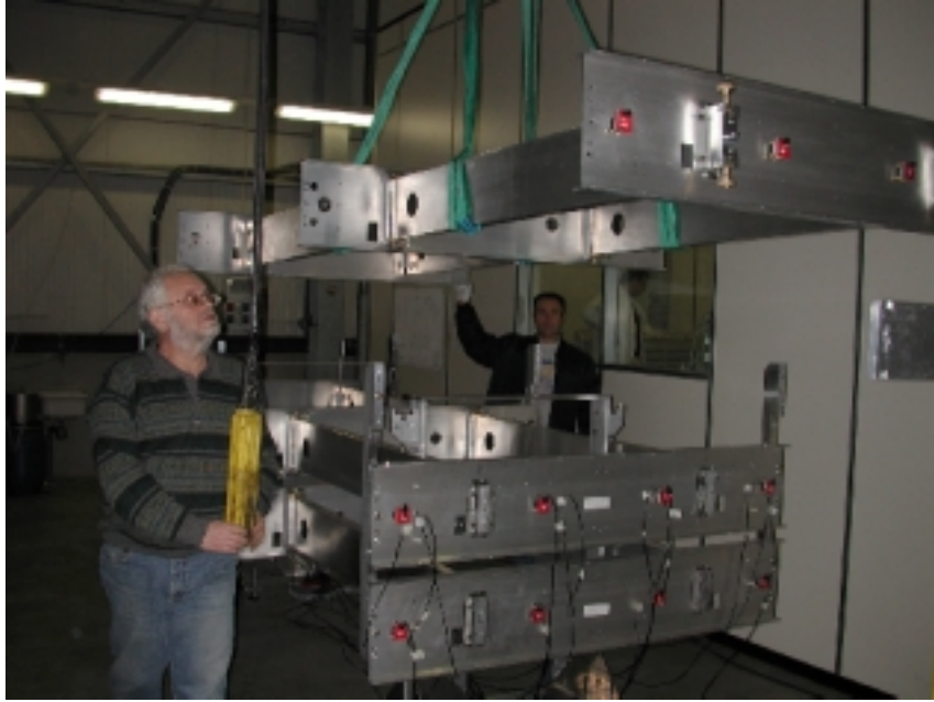
Figure 5: The set-up for the construction of the spacers. The new spacer is glued upon a high precision structure, based of two identical spacers built on a precision granite table.
