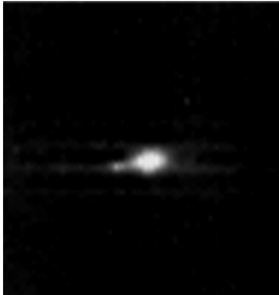
Figure 3: Image of photoelectron track at the focal plane of CCD. It is evident the head of the track less bright carrying the polarization information, followed by a large and bright tail due to a higher energy loss of the photoelectron at the end of the path.
