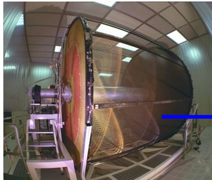
Stereo geometry, 4m diameter
