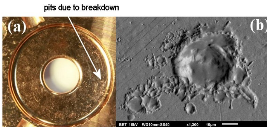
Figure 15. (a) picture of the first accelerating cell, (b) SEM image of craters due to breakdown.
