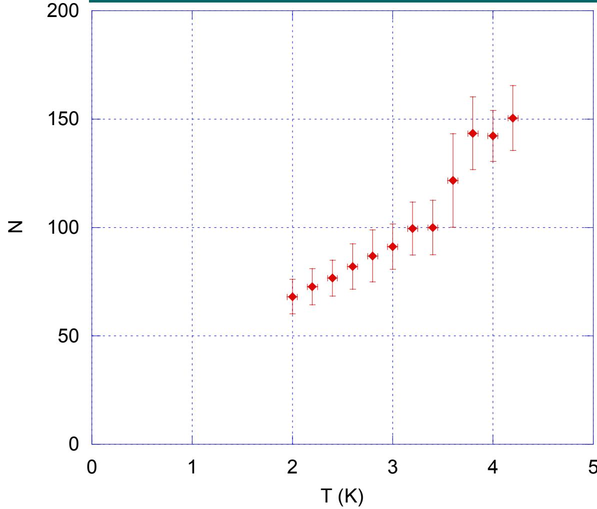
@  $T=2.0$  K, the flux noise is  $0.21\mu\Phi_0/\sqrt{\text{Hz}}$
