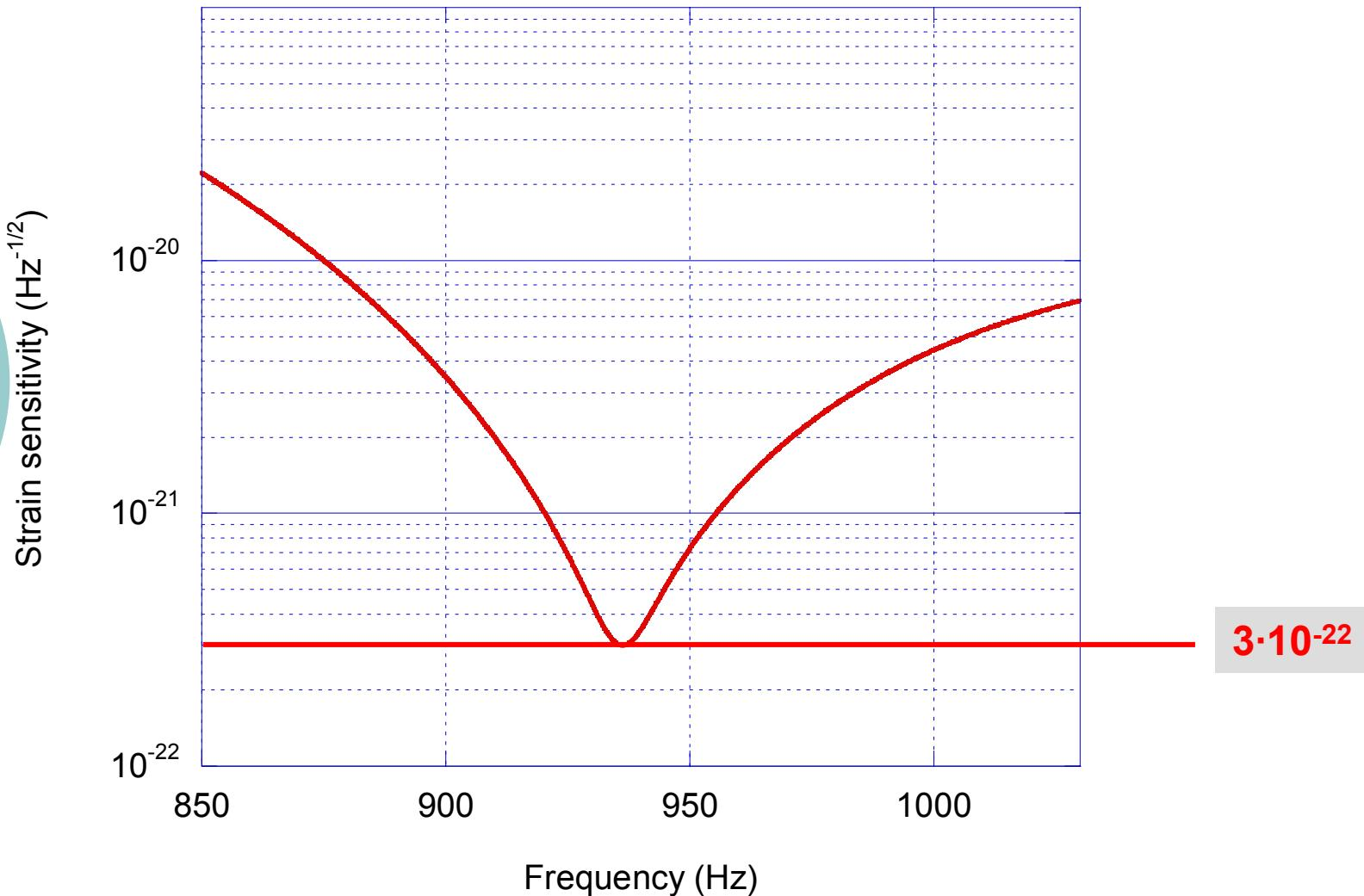
Expected  $S_h$  for NAUTILUS @ 0.12K, double gap transducer (11  $\mu\text{m}$  and  $Q=1.5 \cdot 10^6$ ) and double SQUID ( $L_0=2.5$  H,  $k=0.7$ ,  $\Phi_n = 0.16\mu\Phi_0/\sqrt{\text{Hz}}$ ).
