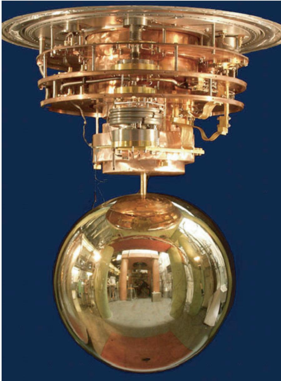
Figure 5.1: The MiniGRAIL detector. The picture shows the last stages of suspension system and of the dilution refrigerator.
