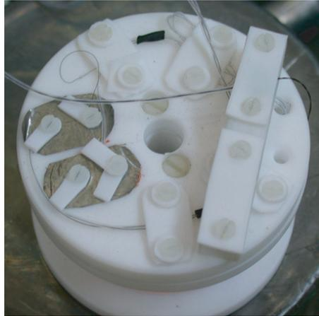
Figure 3.6: Picture of the transformer before insertion in the PVC box. It is possible to notice the weldings on the primary coil.
