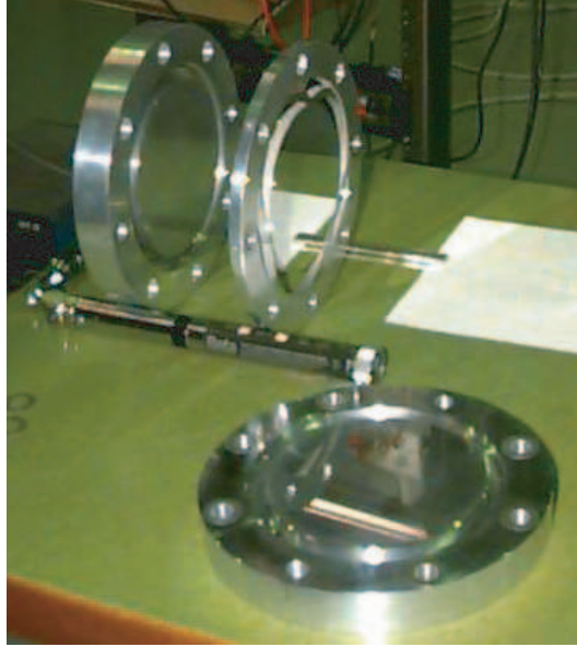
Figure 1. A picture of the double-gap transducer. It is possible to see the two electrodes and the resonator.
