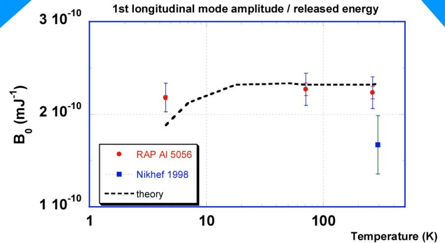
A systematic error of 7% (quadrature beam monitor (3%) + calibration (6%) accuracies) affects the measurements
