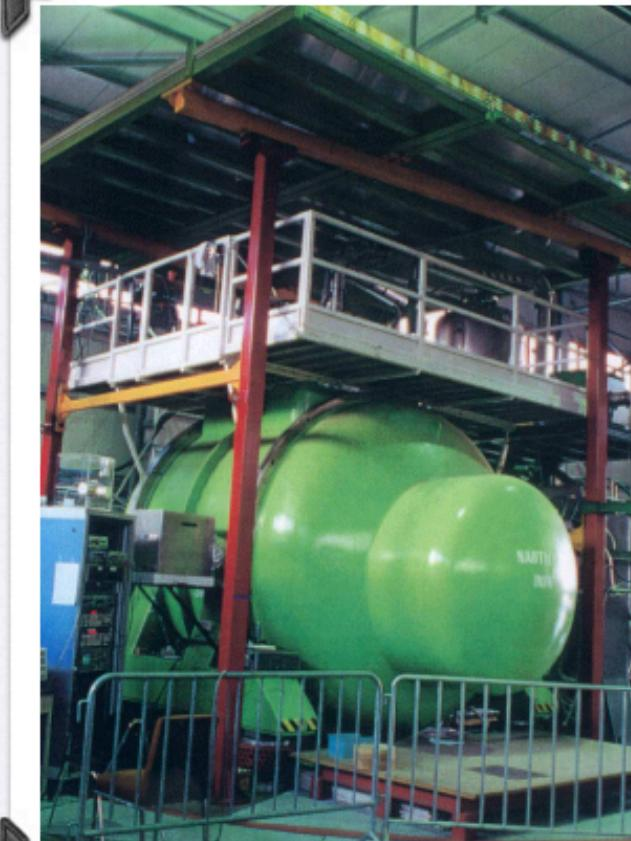
*The NAUTILUS G.W detector has recorded signals due to the passage of cosmic rays.*
