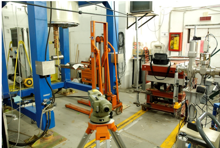
Figure 1. Recent installation of the RAP detector in the DAΦNE Beam Test Facility hall. The mechanical structure, the upper part of the cryostat, as well as the suspension system and the bar are visible on the left side of the picture.
