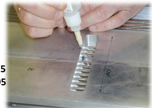
Glueing of straw layer p. 5
