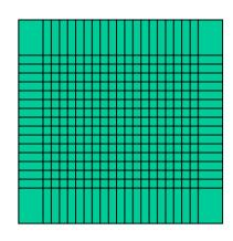
Cover the small size RPC with 48 + 48 strips In order to get a central region of 50x50 cm2 To be used for trigger+tracking (x,y views)
