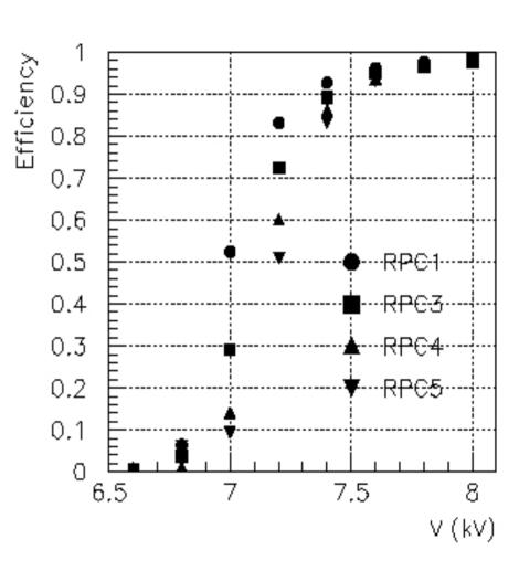
Efficiency curve taken end of August (P=964mbar T=26 C)
