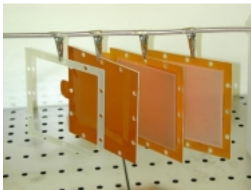
Fig. 3. The three GEMs glued on the G10 frames of different thicknesses.
