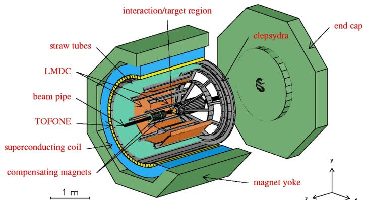
Figure 1: Sketch of the FINUDA apparatus.
