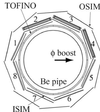
Fig. 1. The FINUDA vertex-target region. The Be pipe, the inner thin scintillator barrel (tofino), the ISIM and OSIM Si-microstrip detectors and the eight targets (numbered from 1 to 8) between them are shown. The bold arrow indicates the direction of  $\Phi$  boost.
