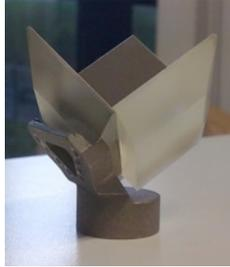
**Figure 5. NASA-GSFC Hollow retroreflector tested at INFN-LNF**
