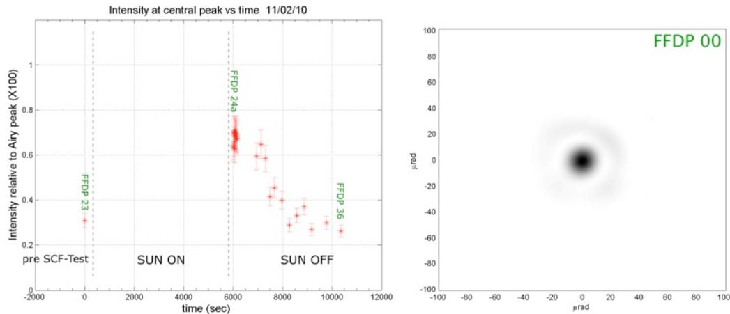
Figure 7. Intensity variation of FFDP at the central peak during the SCF-Test(left). FFDP in air-room temp (right)
