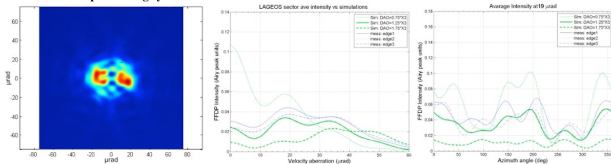
**Figure 2. Left: edge 1 FFDPs . Center: average intensity vs distance from FFDP center. Right: Intensity along a circle at  $19 \mu\text{rad}$ . Comparison between simulated patterns (CODEV) and measured patterns. Measured intensity has  $\pm 25\%$  relative error not shown**
