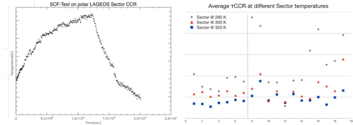
**Figure 3. Left: SCF-Test performed on polar CCR with Sector held at 300K. Right: average  $\tau_{CCR}$  for all of the CCR at various Sector temperatures.**
