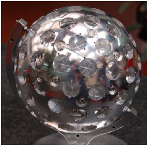
Fig. 10. 1:2 scale prototype of the new shell-over-the-core LARES design built at LNF.
