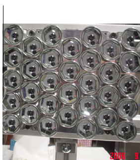
Fig. 2. Left: the third GPS flight CCR array SCF-Tested at LNF. Right: GPS/GIOVE laser returns recorded by the ILRS station at Graz, Austria (courtesy of G. Kirchner).
