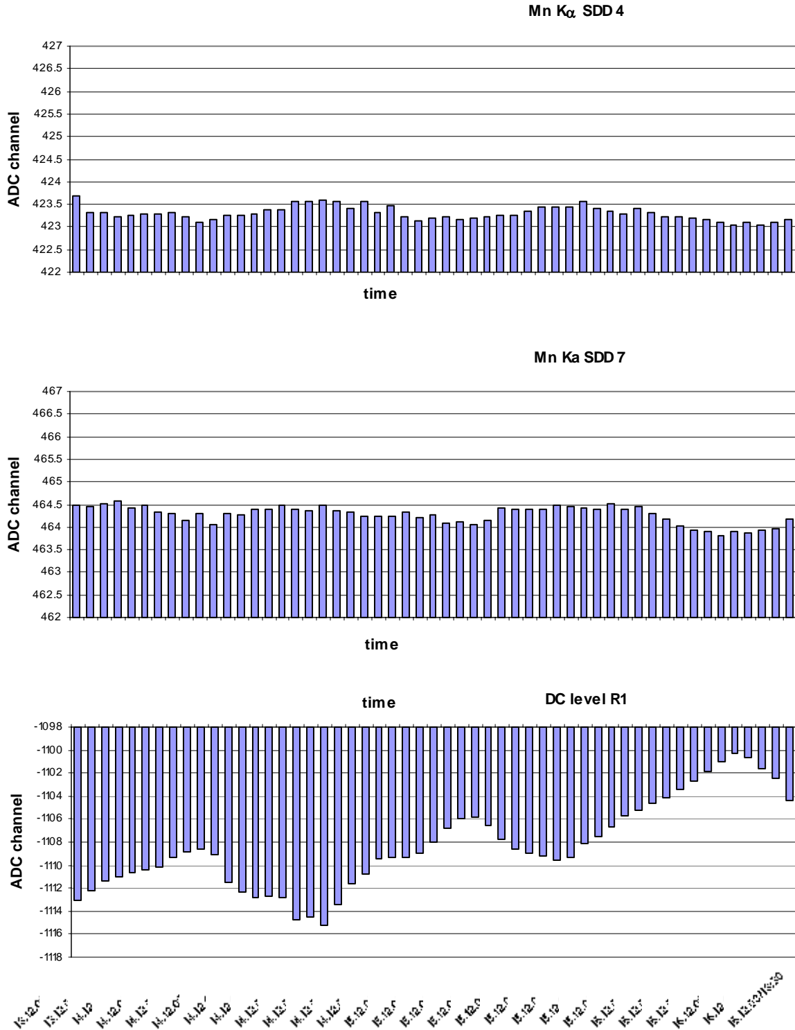
Fig. 4 Mn K\alpha peak position on SDD 4 and 7 and R1 bias voltage
