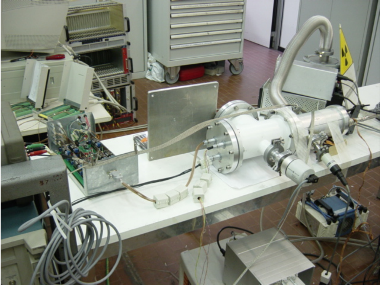
Figure 12: The test setup laboratory tests: detail of readout system is seen
