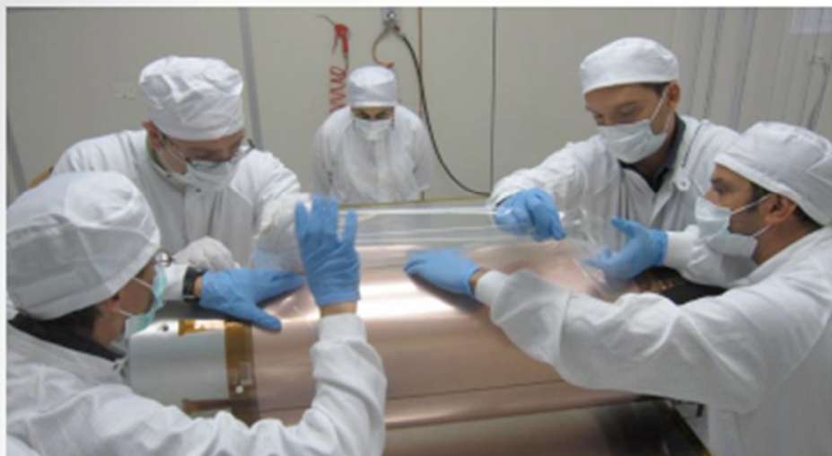
GEM is protected with a Mylar sheet and wrapped on the cylindrical mold
