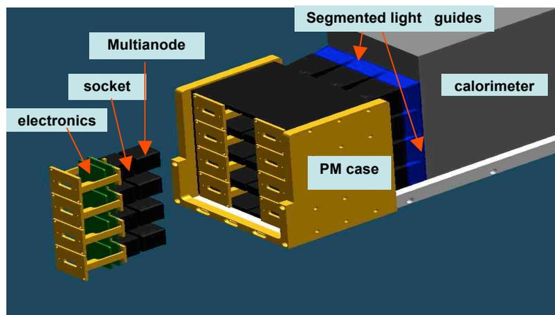
**Figure 6.** Mechanical sketch of the readout support structure (here only 4 PM rows are showed, instead of the final 5)
