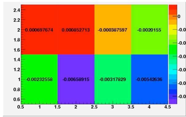
**Figure 8.** Typical response pattern when a single cell is illuminated in an individual multi-anode PM. On both axis the scale is simple cell numbering.
