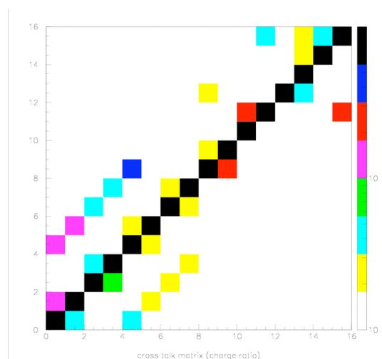
**Figure 4.** Cross talk matrix for a single R8900 at 800 V. Illuminated cell on the x
