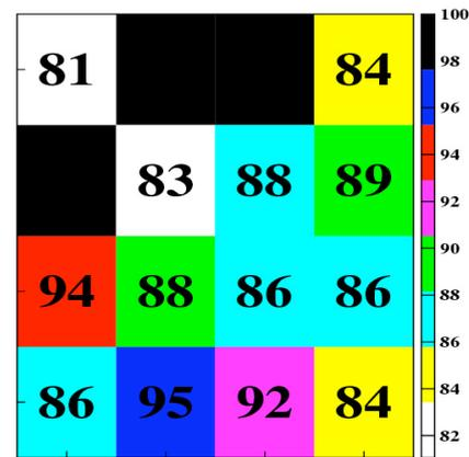
**Figure 3.** Charge response variation at HV=800 V in a typical R8900.
