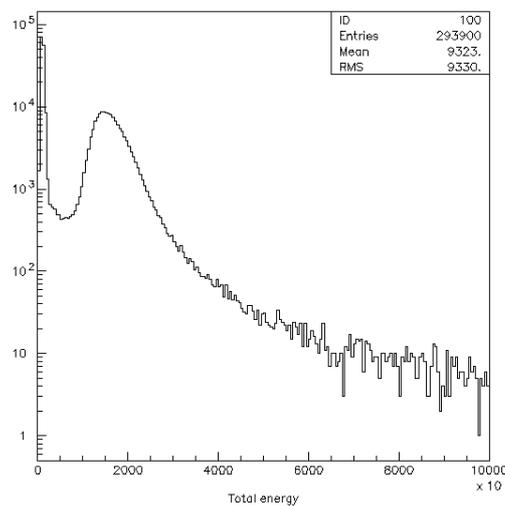
**Figure 11.** Offline sum of all the cells above threshold in the calorimeter over 15000 cosmic rays events.
