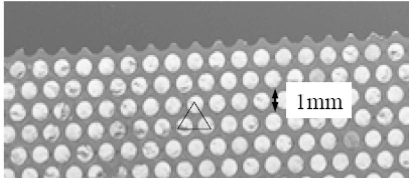
**Figure 1.** Lead- scintillating fibers structure in the KLOE calorimeter.
