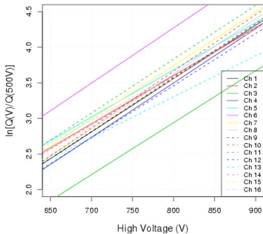
**Figure 2.** Charge response as a function of high voltage for the 16 anodes of a single R8900 M16. Only the fits are shown to save space.
