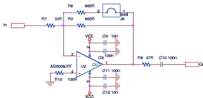
**Figure 7.** Inverting preamplifier stage for a single multi-anode channel.
