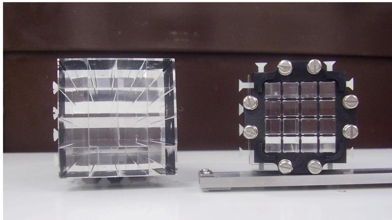
**Figure 5.** View of two blocks of 16 light guides, one seen from the side to be glued to the calorimeter, the other seen from the side to be put in optical contact with the R8900.
