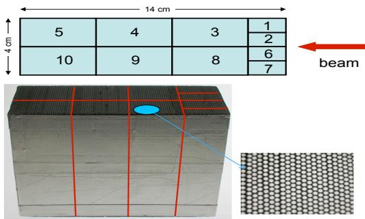
Figure 3: Longitudinal and transversal ZDD module segmentation.
