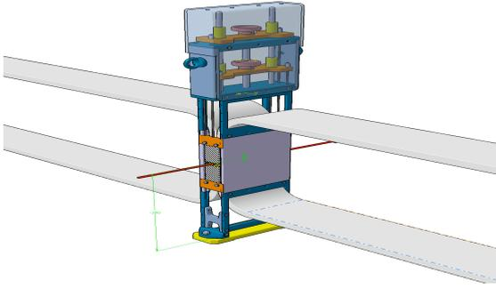
Figure 2: Cartoon showing the ZDD detector mechanical structure used to move the two modules in the vertical direction, to clear the region of maximum bremsstrahlung yield. The four bundles of clear plastic fibers, 2 m long, glued to the modules, to transfer light to the PM's, are also shown.
