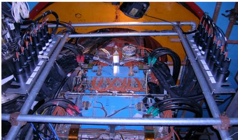
Figure 4: The ZDD detector installed at 3.5 m from the BESIII interaction region, along one of the beam pipes. The ZDD gearbox for vertical movement and the clear fiber bundles connected to the PM's can be seen among many BEPCII accelerator cooling devices.
