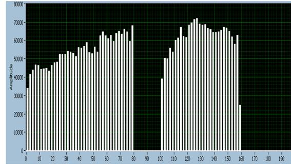
Figure 6: BEPCII bunch structure as seen with the ZDD detector.
