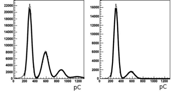
Figure 5: Total charge distribution with 450 MeV electrons ( left plot ) showing clean 1, 2, 3 electron peaks. When the signal is taken in coincidence with the finger counter described in the text, a background free calibration point is obtained (right plot).
