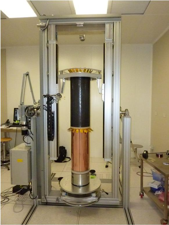
**Figure 3.7:** Two electrodes fixed on the vertical insertion system used to assembly the KLOE-2 detector.
