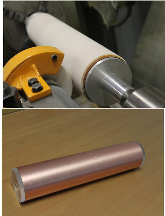
**Figure 3.5:** Top: machining of the Rohacell during the fake cathode construction. Bottom: a picture of the fake cathode with the radius of the innermost layer of the CGEM-IT.
