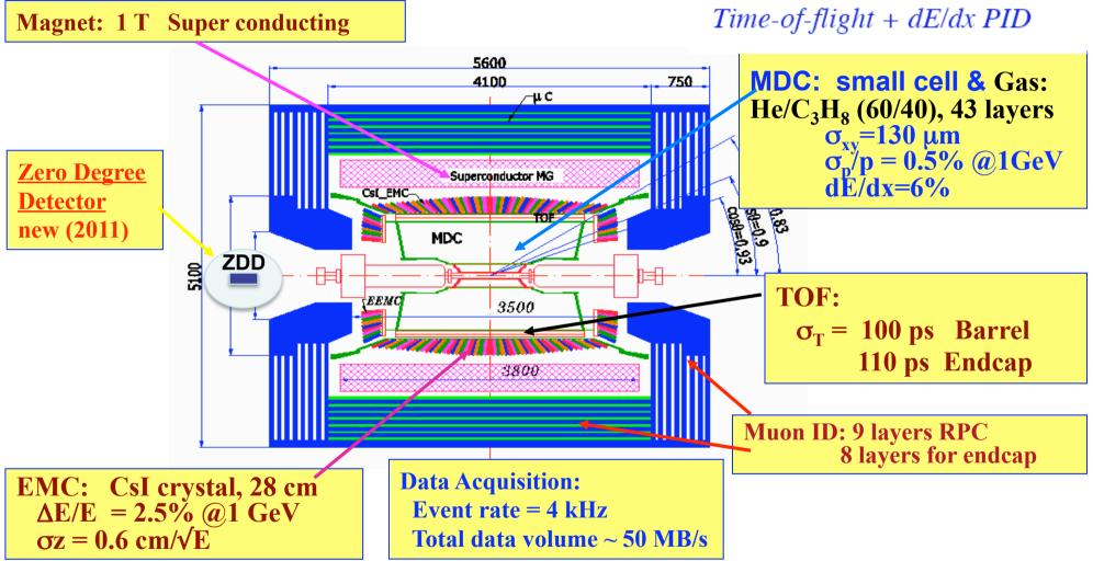
The detector is hermetic for neutral and charged particle with excellent resolution, PID, and large coverage.
