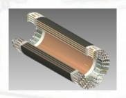
Cylindrical GEM prototype proposal for upgrade of Inner MDC
