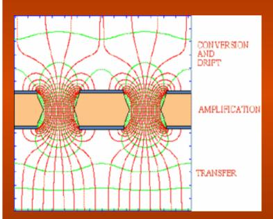
By applying 400-500 V between the two copper sides, an electric field as high as ~100 kV/cm is produced into the holes which act as multiplication channels for electrons produced in the gas by a ionizing particle.
