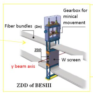
Pb/Sci.Fi Array a` la KLOE scintillating material 60% of total (in volume) two modules (up and down the beam) dimensions:14×4×6cm³ signal extracted and channeled to PM through bundles of clear optical fibers (2m long)
